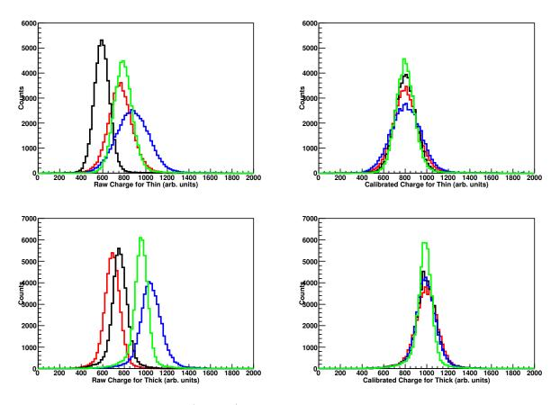
Figure 3.1: Scintillator charge (energy) spectra. The top two plots are from the thin detector, while the bottom two are from the thick scintillator. The events were gated so that only one isotope was present along with the beam being centered in both detectors. The left plots show the raw energy collected while the right plots show the four PMTs after gain matching. The thin and thick LU, RU, LD, and RD are represented by the color red, black, blue and green, respectively.
