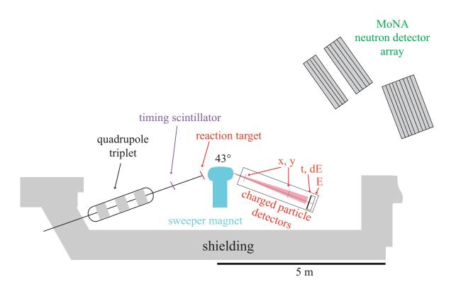
Figure 2.2: Diagram of the experimental vault. It shows the placement of the target, quadrupole triplet, Sweeper magnet, and the detectors.
