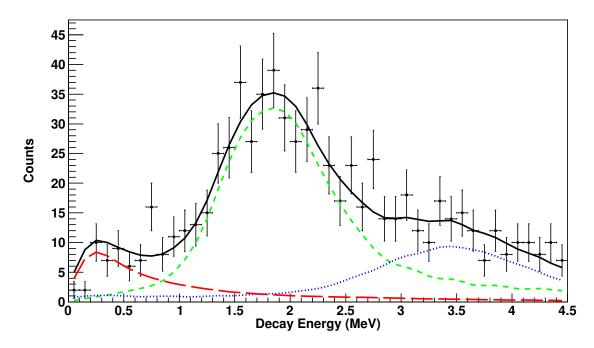
Figure 5.1: <sup>15</sup>Be decay energy spectrum. The data are shown by the black data points with statistical error bars. The best fit to the data (solid black line) is a sum of an l = 2 resonance (green short-dashed line) and background contributions approximated by l = 0 (red long-dashed line) and l > 0 (blue dotted line) components.
