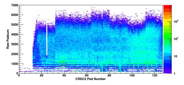
Figure 3.4: CRDC2 raw charge collected values for each pad from a sweep run that illuminated the entire face of the detector.
