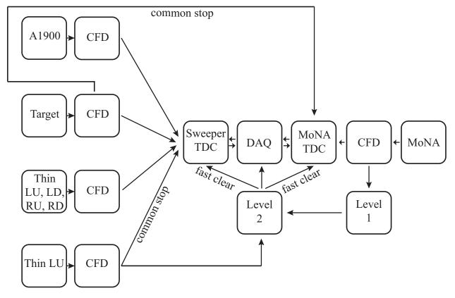
Figure 2.4: Schematic diagram of the timing electronics, logic modules, and DAQ. If there is a valid event in MoNA, the Level 1 logic module sends a signal to the Level 2 logic module which waits for a signal from the thin LU to determine if there is a valid coincidence. If there is a valid coincidence, Level 2 sends a signal to the DAQ to read out all of the electronics. If there is no coincidence in the Level 2 sends out a signal to fast clear the electronics.
