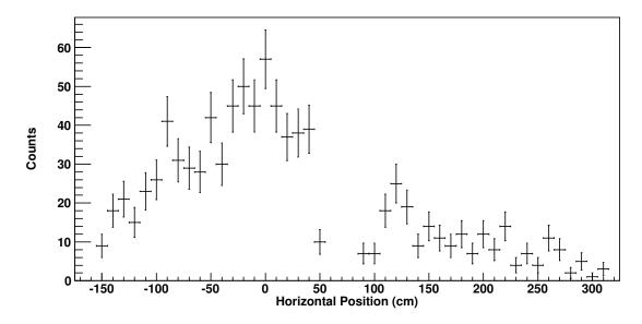
Figure 3.20: The horizontal distribution of neutron events in MoNA from the formation of <sup>15</sup>Be by neutron pick–up from the target.
