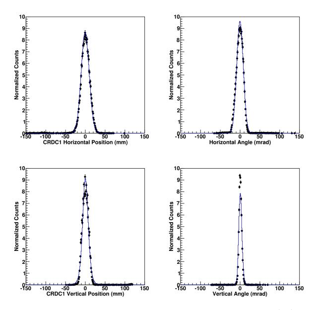
Figure 4.1: CRDC position and angle spectrum. Each figure compares data (dot) to ST MoNA simulation (line). The top left, top right, bottom left, and bottom right panel shows the comparison for the CRDC1 horizontal position, horizontal angle, vertical position, and vertical angle, respectively.
