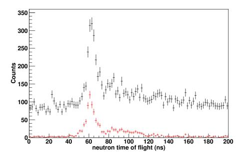
Figure 3.19: Neutron time of flight spectrum. The black data points represent the time of flight for <sup>14</sup>Be fragments that were selected using the gate shown in Fig. 3.16. The red data points have an additional gate on deposited energies of more than 3 MeVee.
