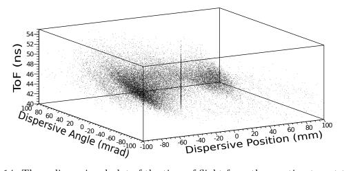
Figure 3.14: Three dimensional plot of the time of flight from the reaction target to the thin scintillator vs. dispersive angle at the focal plane vs. dispersive position at the focal plane. The plot only contains beryllium isotopes. The bands correspond to different isotopes with the most intense being <sup>14</sup>Be.
