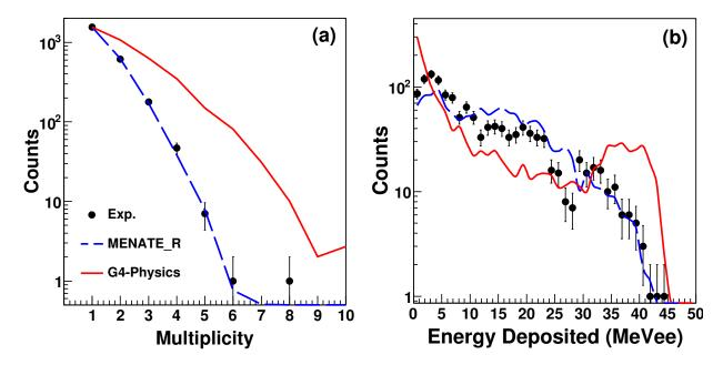
Figure 4.10: Experimental data (Black) from Ref. [77] is compared to the G4Physics (Red) and Menate\_R (Blue) model. The left panel shows the multiplicity and right panel shows the energy deposited. In the left panel the multiplicity distributions were normalized so that multiplicity = 1 events matched. The right panel was normalized for total number of events. (adopted from Ref. [79])
