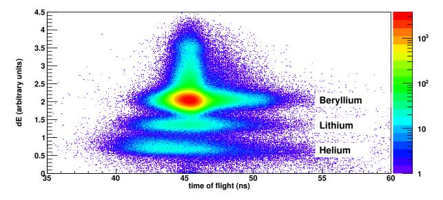
Figure 3.13: Element identification is determined using the time of flight between the target and thin plastic scintillator vs energy loss in the thin plastic scintillator. The elements present are identified in the plot.
