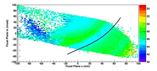
Figure 3.15: Projection of Figure 3.14 where the color corresponds to time of flight between the reaction target and the thin scintillator. A band of equal time of flight is fitted to construct a parameter describing the correlations between the dispersive angle and position.
