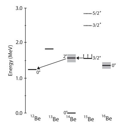
Figure 1.2: Level scheme for neutron rich beryllium isotopes. The solid lines indicate experimentally known levels with the uncertainties being represented by the gray squares, whereas the dashed lines come from NUSHELLX calculations using the WBP Hamiltonian. The arrows show the decay path taken from the population of the  $3/2^+$  state as determined from Ref. [17].
