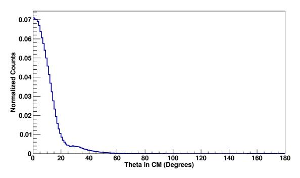
Figure 4.4: Angular distribution of the reaction used in ST MoNA, calculated with FRESCO using the global optical potentials from Refs. [38, 35].
