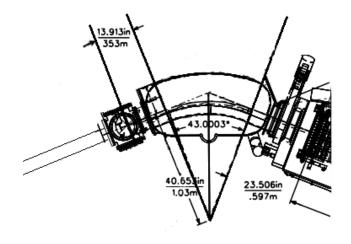
Figure 4.2: A technical drawing of the beam–line from the target to the focal plane box. The central track length from the target to CRDC1 can be determined using this diagram.
