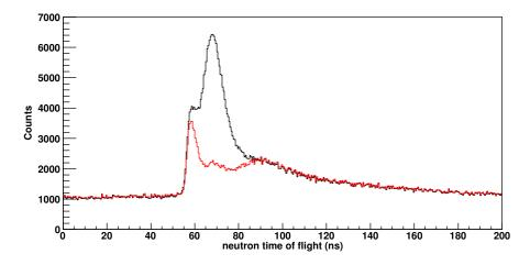
Figure 3.18: Neutron time of flight spectrum. The black data points represent the time of flight for all beryllium isotopes whereas the red data points are in coincidence with  $^{14}$ Be fragments.
