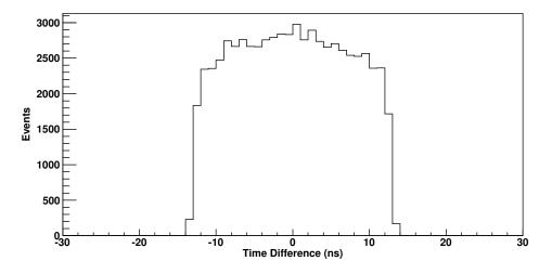
Figure 3.10: Example time difference between the right and left sides of a bar from a cosmic muon run. The edges of the bar are easily identified which allows for a linear calibration to determine the slope and offset. This allows for the determination of where the event took place.
