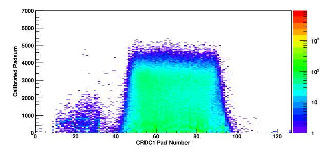
Figure 3.6: CRDC1 calibrated charge collected for each pad from a sweep run that illuminated the entire face of CRDC2. The pedestals have been subtracted, and each pad has been gain matched. The color represents the number of counts per bin.
