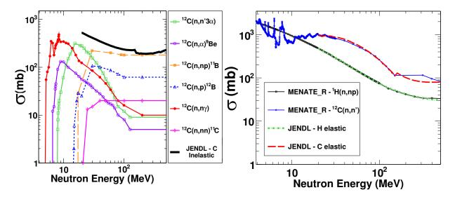
Figure 4.8: The left panel shows the total carbon-neutron inelastic reaction cross section used in the stock G4Physics class (JENDL-HE). The other six colors show the discrete inelastic reaction cross sections used in the Menate\_R code. The right panel shows the hydrogen elastic cross section for G4Physics Class (Green) and Menate\_R (Black). Also shown is the carbon elastic cross section for the G4Physics (Red) and Menate\_R (Blue). (adopted from Ref. [79])
