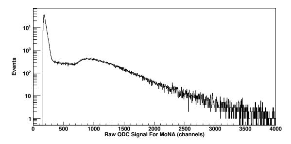
Figure 3.9: Example raw QDC spectra for a single MoNA PMT. The cosmic muon peak can be seen at approximately channel 900, room  $\gamma$ -rays are located at channel 250 and the pedestal is not present since it has been already suppressed. For the linear calibration the pedestal was set to zero and the centroid of the cosmic muon peak was set to 20.5 MeVee.
