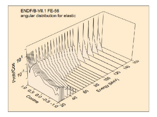
Figure 4.9: Visual representation of the elastic cross sections for iron at different energies from Ref [78]. The cross sections at 30, 50, and 70 MeV were added to Menate\_R, and then extrapolated to the energy of the neutron.
