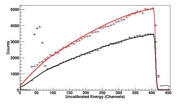
Figure 5.3: RBS simulations using 3.4 MeV protons impinging upon a carbon (red line) and a CH<sub>2</sub> (black line) target are compared to data from RBS analysis, also using 3.4 MeV protons. The carbon data (red points) and deuterated polyethylene data (black points) were normalized to the simulated carbon target. There is good agreement between the simulated deuterated polyethylene target and the data, which indicates that the ratio of carbon to hydrogen is 1:2.
