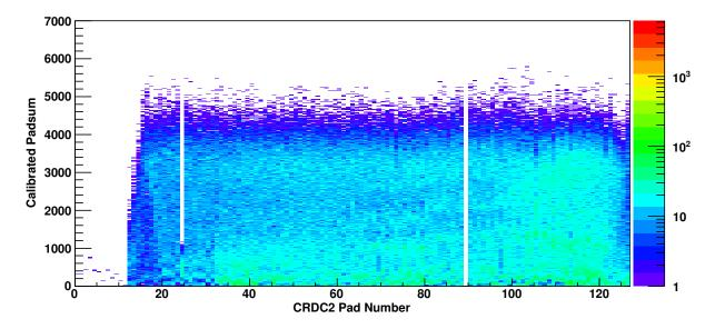
Figure 3.5: CRDC2 calibrated charge collected for each pad from a sweep run that illuminated the entire face of CRDC2. The pedestals have been subtracted, and each pad has been gain matched.
