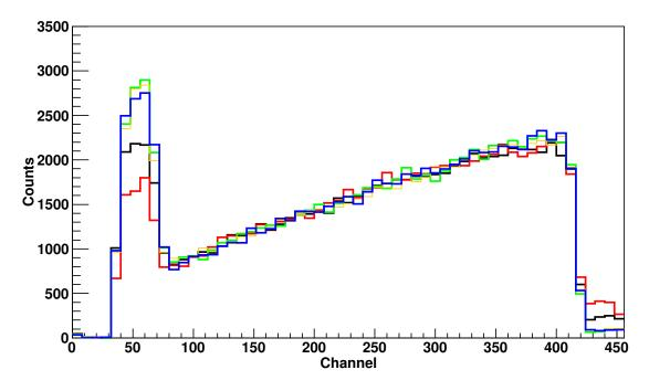
Figure 5.4: RBS data for five different locations on the deuterated polyethylene target, impinged with 3.4 MeV protons. Each data set was normalized so the total number of incoming protons were the same. The strength of the peak between channel 30 and 70 is indicative of the percentage of hydrogen in the target is deuterium.
