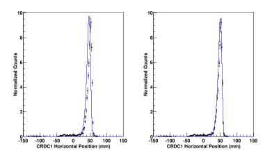
Figure 4.3: Experimental and simulation data obtained with the Sweeper magnet's current at 366 A. The blue line represents an ST MoNA simulation, while black points represents experimental data. The left panel reflects a simulated total central track length of 165.4 cm and the right panel uses 172.3 cm.
