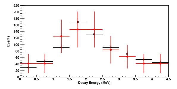
Figure 3.24: Decay energy spectrum for deuterated polyethylene and a carbon target. A 300 mg/cm<sup>2</sup> carbon target was used for 16 hours, the decay energy for the carbon target (red data points) is compared to the deuterated polyethylene target (black data points). The gates and conditions used to select and calibrate for both targets were the same and the results are statistically identical.
