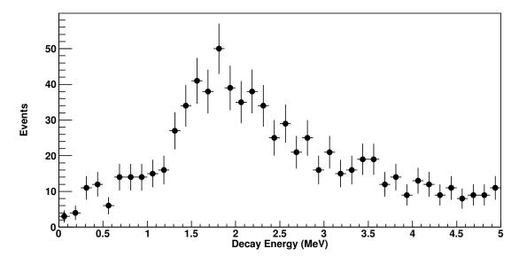
Figure 3.23: Decay energy spectrum for coincidence <sup>14</sup>Be and a neutron is shown by the black data points with their statistical uncertainty. The spectrum was calculated using Eq. 2.6. A resonance can clearly be seen at approximately 2 MeV.
