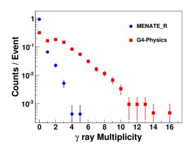
Figure 4.11: Comparison between the stock G4Physics (Red) and Menate\_R (Blue) models of multiplicity distribution for interactions within MoNA where  $\gamma$  rays are produced from inelastic reactions with carbon. (adopted from Ref. [79])
