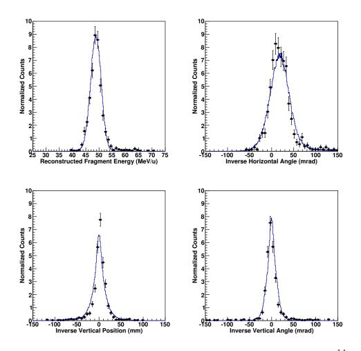
Figure 4.6: Comparison of simulation (blue line) to data (black points) for <sup>14</sup>Be reaction products located in the focal plane. The parameters are compared are target E,  $\Theta_X$ , Y, and  $\Theta_Y$  which are located in the upper–left, upper–right, lower–left, and lower–right panel, respectively.
