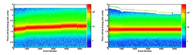
Figure 3.2: Uncorrected thick left-up energy (left panel) and after the time correction factor has been applied (right panel) plotted against event number. The correction factors were determined for each of the PMT for the thin and thick scintillators.
