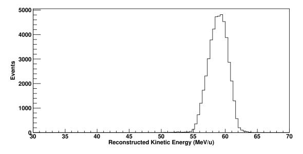
Figure 3.21: Reconstructed kinetic energy spectrum which is used to test the inverse map. The data comes from a no target run that was bent into the center of the focal plane box. The reconstructed energy is in complete agreement with the value predicted by LISE++ of 59 MeV/u
