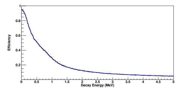
Figure 4.7: Geometric efficiency of the MoNA and Sweeper system. It was calculated for energies between 0 and 5 MeV for a neutron pick–up reaction from deuterium.
