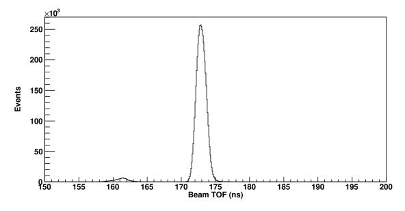
Figure 3.11: Flight time for the incoming beam from the A1900 timing scintillator to the target scintillator. The <sup>14</sup>Be is centered around 173 ns, with the biggest contaminant coming from lithium which is centered at 161.5 ns.
