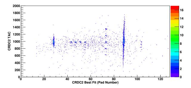
Figure 3.7: Example mask run for CRDC2. The best fit (pad number) is plotted vs TAC. The holes are easily identifiable and gates were applied around each one and the centroid a gaussian was used to find the centroid in TAC and best fit (pad number).
