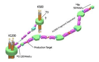
Figure 2.1: Diagram of the beam production mechanism. The primary beam of  $^{18}$ O is accelerated through the K500 and K1200 until it reaches an energy of 120 MeV/u and strikes a 3196 mg/cm<sup>2</sup> beryllium target. The A1900 fragment separator then selects  $^{14}$ Be fragments from other reaction products.
