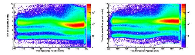
Figure 3.3:  $\Delta E$  from the thin scintillator (left panel) and corrected  $\Delta E$  (right panel) is plotted against the horizontal position of the detector. The correction is Z dependent, thus it only straightens the beryllium band.
