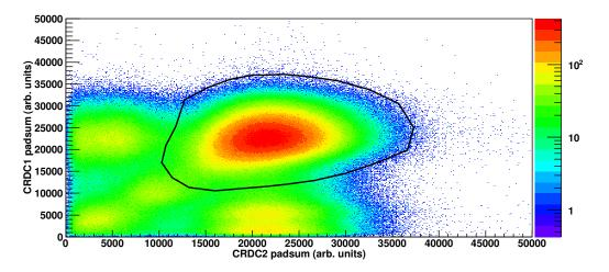
Figure 3.12: CRDC1 padsum plotted against CRDC2 padsum. No gates were applied to this plot. The black line corresponds to the gate used to select for good padsum in CRDC1 and CRDC2.
