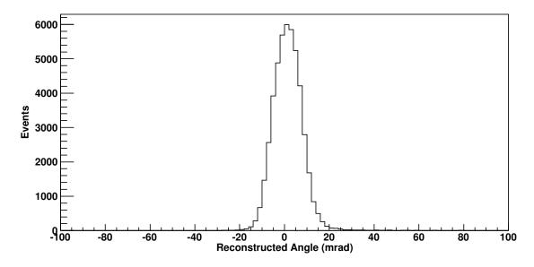
Figure 3.22: Reconstructed angle spectrum that is used to test the inverse map. The data comes from a no target run that was bent into the center of the focal plane box. The reconstructed angle is centered, confirming that the inverse map is working properly.
