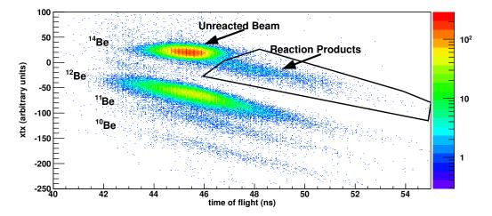
Figure 3.16: The parameter xtx versus time of flight between the reaction target and the thin scintillator. Isotopes are identified on the plot, along with where the unreacted beam and reaction products are located for <sup>14</sup>Be. The black line corresponds to the gate used to remove contamination of unreacted <sup>14</sup>Be. In order to reduce the intensity of the unreacted beam, a gate on beam velocity neutrons in MoNA was applied.
